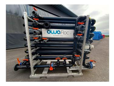
OwaFloc can be connected as part of the OwaMobile chemical treatment or installed separately to enhance existing water treatment. The number of connections has been considered in the unit to be used for dosing and mixing several different chemicals. Solid matter and other impurities can be separated from the water almost entirely by enhancing water treatment with chemical treatment.
