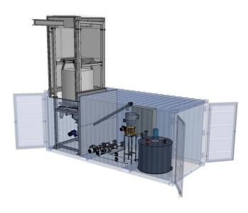
OwaBalance with automated milk of magnesium and limewater preparation and dosing system. The pH adjustment is connected to the dosing, which enables the optimal maintenance of the target values, for example, in the precipitation of metals. Automation guarantees effective processes in areas with challenging circumstances.
