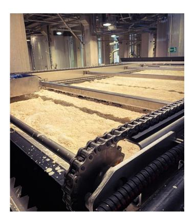
The efficiency of the flotation unit is based on the KTM Bubble Generator – multiphase pump, which feeds micro and nanobubbles that separate solid matter and other impurities to the surface, making traditional dispersion or pure water supply unnecessary. In addition to air, the KTM Bubble Generator pump can feed other gases into the water, such as nitrogen and oxygen.
